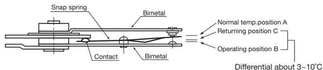
The narrow differential, sharp snap action spring plays an important role in achieving desirable thermostatic response. This snap spring turns on and off over an exceptionally small distance (approx. 0.05mm), or in terms of temperature, approx. 3°C Beryllium bronze snap spring can withstand at least 2 million operations.
