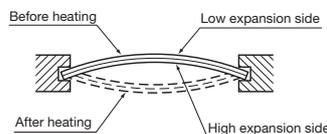
By forming a bimetal strip into a dome shape (hemispherical, dished shape) to acquire snap action, the disk type protector is characterized by its simplicity of construction. The simple design facilitates volume production and, because of its low cost, account for 80% of the entire bimetallic thermal protector market in the world.
