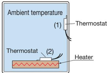
To control the ambient temperature within an enclosure, place a thermostat in position (2) in the figure. A thermostat installed in position (1) cannot provide proper temperature control.
