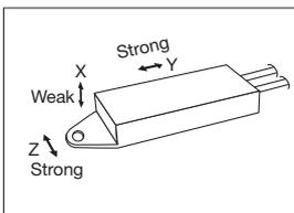
The TPS is delicate to impacts in the X direction and strong in the Y and Z directions (see the figure to the left). When a TPS is dropped from a height of 70 cm to the floor and it sustains an impact in the X direction, a temperature setting error between 2 and 3 may occur.
