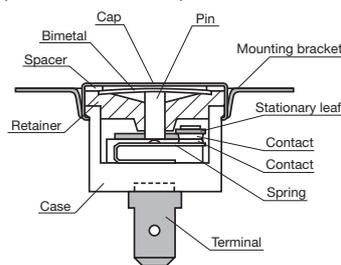
However, the bimetallic material has physical properties similar to ordinary steel material and is not a spring material in itself. During the course of repeated tripping, it is no wonder that just a strip of ordinary metal, formed into a dome, will progressively distort, or lose its shape, and return to its original shape of a flat strip.
